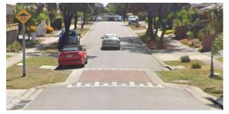
Note: Speed humps and other 'deflection' devices must be located near street lighting to ensure they are visible at night
